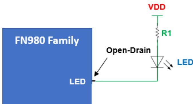
R1 and VDD determine the brightness of LED and forward current.
